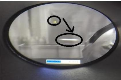
Above, the yellow aiming box isn't over the white flashing beam, in this case it needs to be moved down and right.
