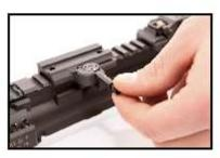
STEP FOUR; TIGHTEN ADJUST-MENT SCREW ALL THE WAY TO LOCK ADJUSTMENT WHEEL IN PLACE.
