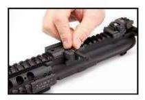
STEP TUREE: TURN ADJUSTMENT WHEEL CLOCKWISE TO TIGHTEN COUNTER CLOCKWISE TO LOOSEN, EACH CLICK IS .002" OF ADJUST-MENT. BE CAUTIOUS NOT TO OVER-TIGHTEN.
