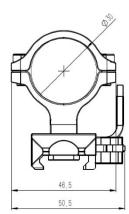
**Note:** Use M6 screws to fix the mount on the riflescopes.
