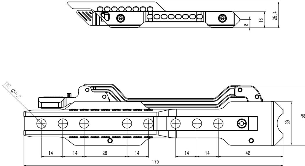
**Note:** Use M6 screws to fix the mount on the riflescopes.
